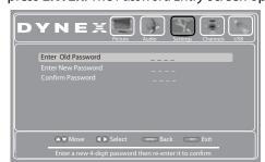
6 Press the number buttons to enter the old password, enter a new password, then enter the new password again. The password has been successfully changed.
